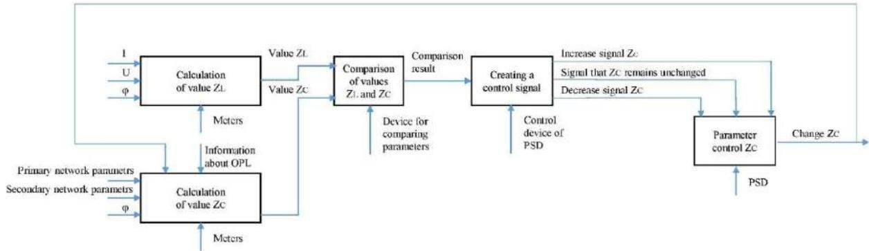
**Fig. 1. Information process diagram for phase-shifting devices**
