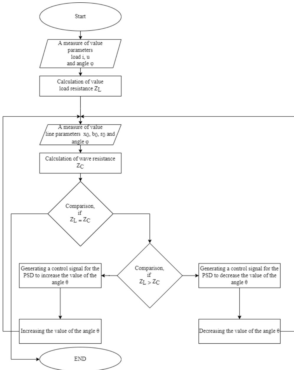
**Fig. 2. Algorithm flowchart for phase-shifting devices in the information-and-control system**
