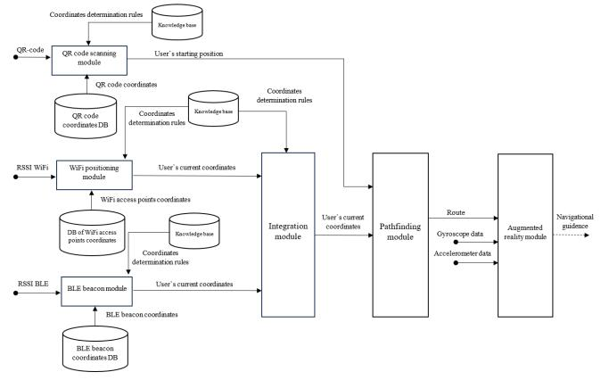
Fig. 2. Model of system component interaction
