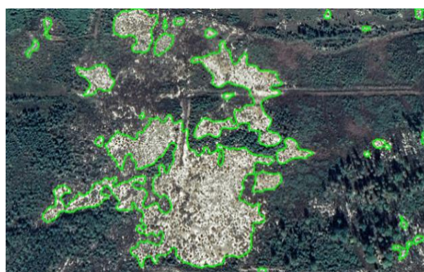
Fig. 7. High spatial resolution digital test aerial photograph highlighting of amber extraction contours using the proposed methodology
