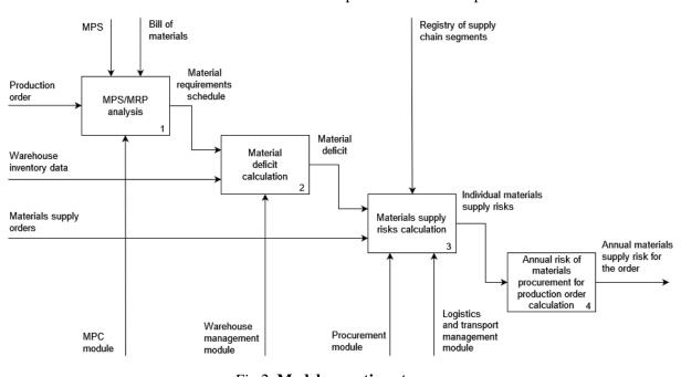
Fig 2. Model execution stages Source: compiled by the authors Let's review the implementation of the model using the example of calculating material supply risks for an order to manufacture VVG 3x2.5 power cable.
