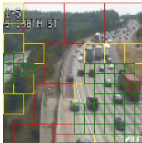
Fig. 6. Adaptive patch grid based on motion intensity Source: compiled by the authors
