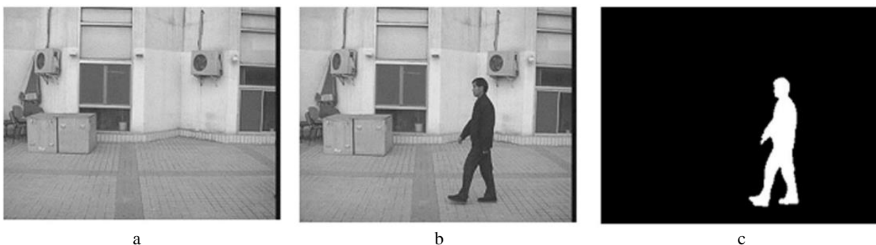
Fig. 1. Example of gait detection: a – Background image; b – original image; c – extracted silhouette
