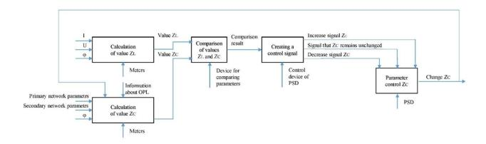
Fig. 1. Information process diagram for phase-shifting devices Source: compiled by the author
