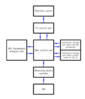
Fig. 3. Functional diagram of the informationand-control system
