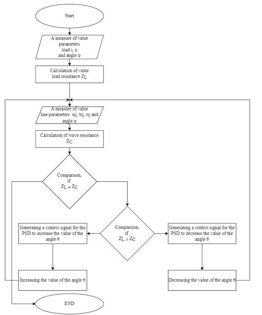
Fig. 2. Algorithm flowchart for phase-shifting devices in the information-and-control system Source: compiled by the author
