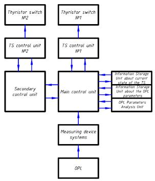
Fig. 4. General functional diagram of the ICS of two phase-shifting devices in one circuit of a double circuit controlled power high-voltage lines
