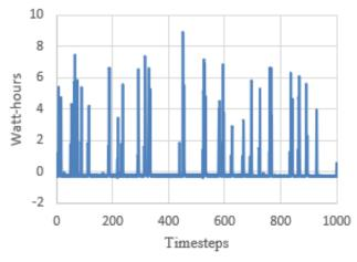
Fig. 5. Graph of active energy consumption of the laundry in the interval 1 to 1000
