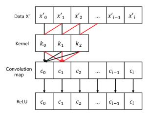
Fig. 7. Operation of a one-dimensional convolution layera
