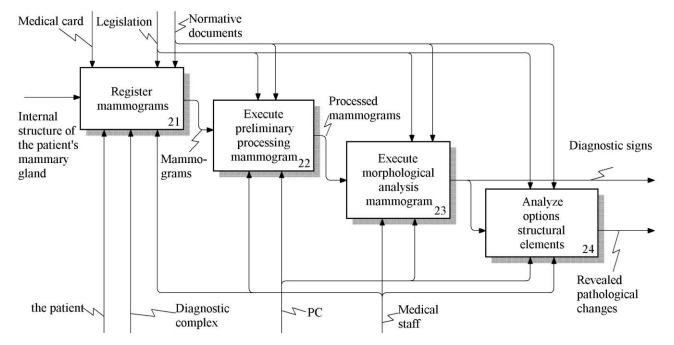
Fig. 3. Decomposition of functional block 2 "Perform registration and analysis of mammograms" of the functional model  $M_F$  mammographic examination Source: compiled by the author
