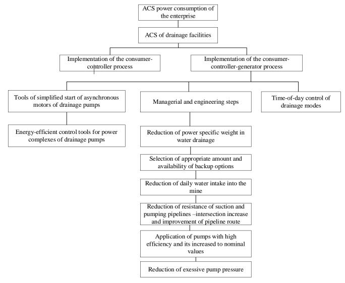
Fig. 1. Basic algorithm of the subsystem ACS of drainage facilities functioning Source: compiled by the authors
