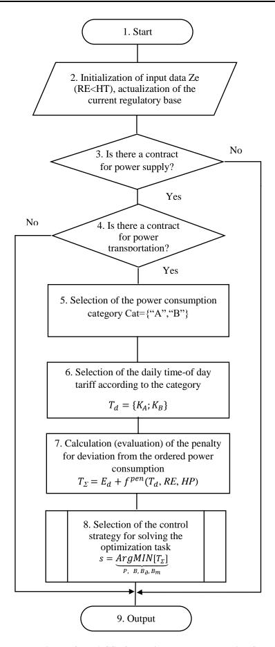
Fig. 2. General algorithm of the ACS of electric power consumption functioning Source: compiled by the authors
