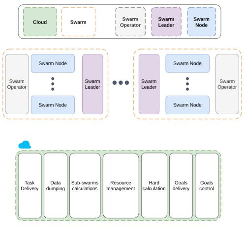
Fig. 5. Swarm Womb logical view and high-level system structure Source: compiled by the authors
