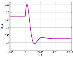
Fig. 21. Excitation current transient process graph in a case of load change Source: compiled by the authors
