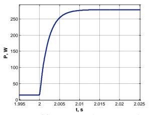
Fig. 20. HESG output electric power transient process graph in a case of wind speed change Source: compiled by the authors
