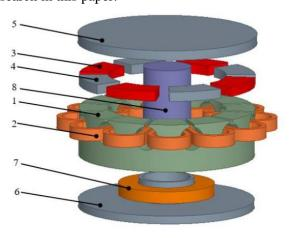
Fig. 1. Axial magnetic flux synchronous generator
