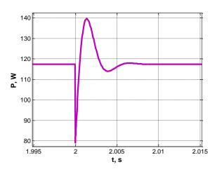
Fig. 22. Maximum output power transient process graph in a case of load change Source: compiled by the authors
