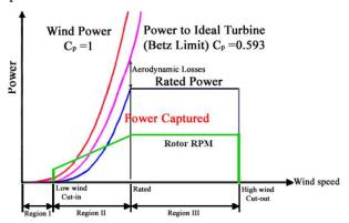
Fig. 2. Turbine output power versus wind speed Source: [4]
