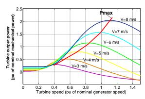
Fig. 6. Mechanical power versus rotation speed of wind turbine for a given experimental HESG Source: compiled by the authors
