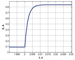
Fig. 19. Field excitation current transient process graph in a case of wind speed change Source: compiled by the authors
