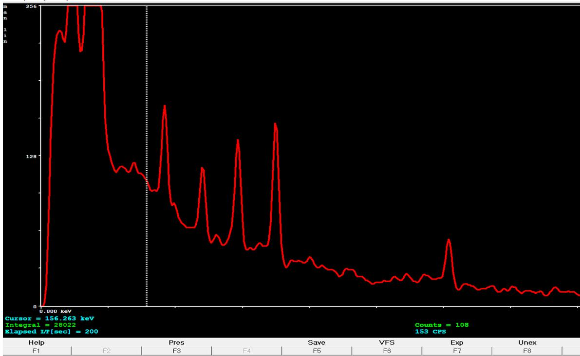
**Fig. 2. Gamma-ray spectra <sup>133</sup>Ba**
