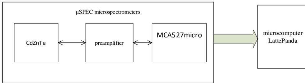
**Fig. 4. CZT-spectrometer operation**
