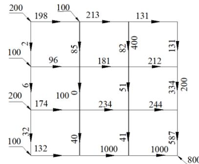
Fig. 7. An example of numerical calculations of the optimal network load
