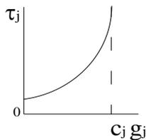
**Fig. 2 Dependence of the message transmission time on the intensity of the information flow**
