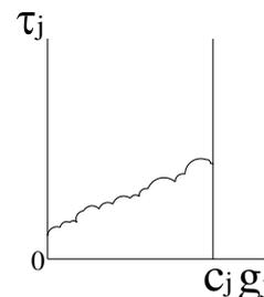
**Fig. 4. Approximation of the information transfer time by a step function**
