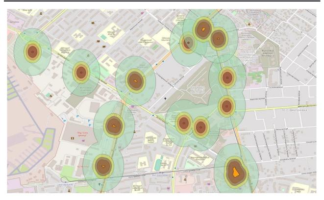
*Fig. 5.* Visualization of risk zones from gasoline tanks of filling stations with maximum capacity (40 m<sup>3</sup>) in one of the residential districts of the city of Odessa *Source:* compiled by the author
