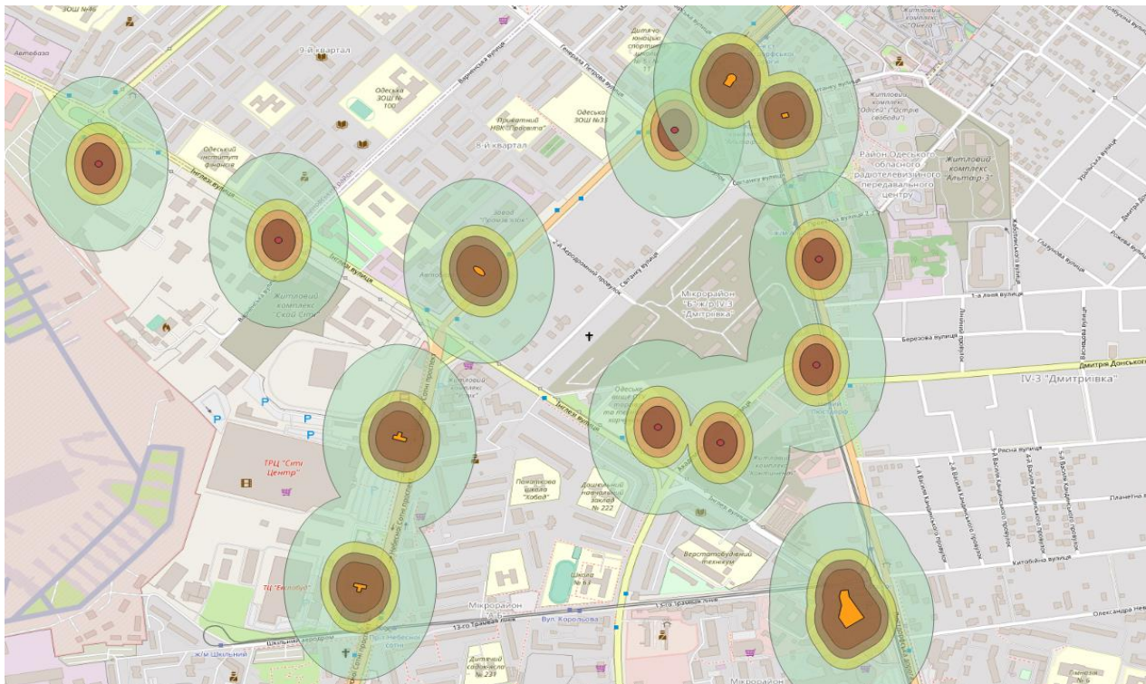
Fig. 5. Visualization of risk zones from gasoline tanks of filling stations with maximum capacity ( 40 \text{ m}^3 ) in one of the residential districts of the city of Odessa
